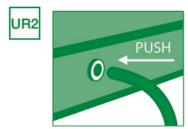
Use a step drill bit to drill a 12mm / 1/2" dia. hole in your reservoir. Push the 3/8" grommet into your reservoir. Push 3/8"pipe through grommet.
