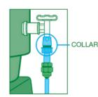
reservoir tap. If your tap is not Click-Fit remove the collar from the Filter and push pipe directly onto tap.
