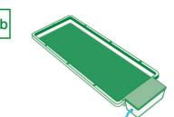
Wet and lay root control sheet on top of capillary matting. The root control sheet can be laid copper side up or down.
